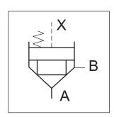
The basic element incorporated in both the body mounted and cartridge type (manifold) mounted series is the main cartridge comprising poppet spool, sleeve and spring. The wide range of optional combinations are based on an integrated system which offers easy modification to existing circuits incorporating the Veljan Seat valve/cartridge modules. Close manufacturing tolerances permit simple change or addition without special fitting.
