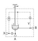
VD4S\*\*-\*23-3B\* with stroke limiter Pilot oil X = external Note: for VD4S06 & VD4S10 only
