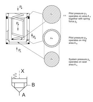
Example: With a ratio of 95% seat area to 5% ring area and a spring pressure = 2.2 bar then the following cracking pressures apply.
