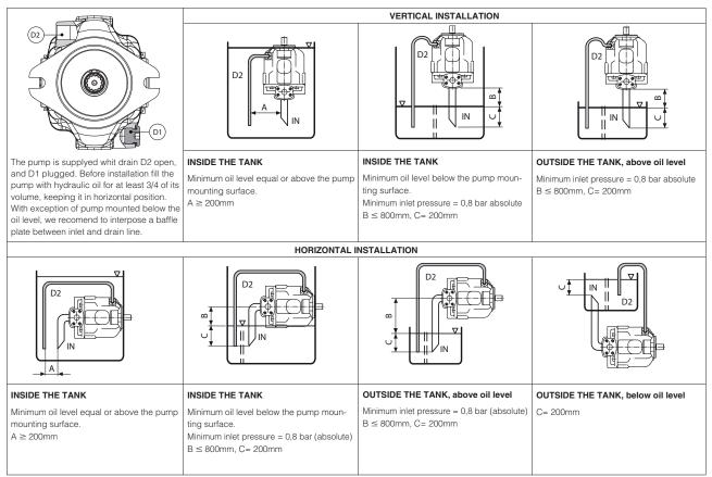
IN: inlet line - D2: drain line - A: minimum distance between inlet and drain line - B+C: permissible suction height - C: inlet line immersion dept
