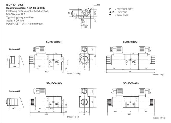
Overall dimensions refer to valves with connectors type SP-666
